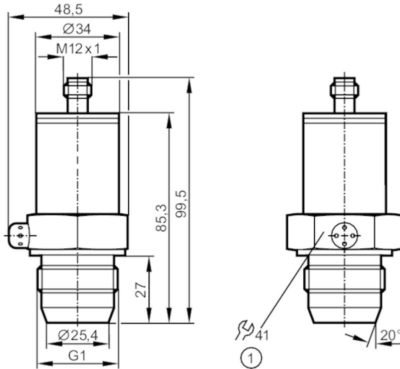
1 Tightening torque 20 Nm
