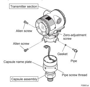
Figure 9.5 Removing and Mounting the Capsule Assembly
