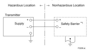
\*1: In any safety barriers used the output current must be limited by a resistor "R" such that Imaxout-Uz/R.
