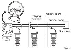
Figure 8.1 Connecting the BT200
