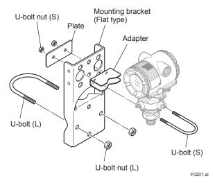
Figure 2.1 Transmitter Mounting Hardware
