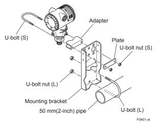
Figure 4.1 Transmitter Mounting
