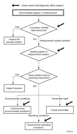
Figure 9.6 Basic Flow and Self-Diagnostics
