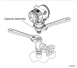
Figure 4.3 Tightening Transmitter
