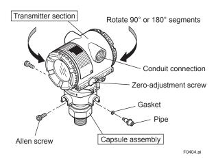
Figure 4.4 Rotating Transmitter Section
