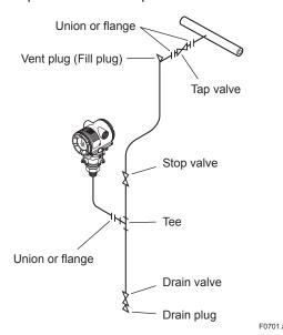
Figure 7.1 Liquid Flow Measurement (Gauge Pressure Transmitters)
