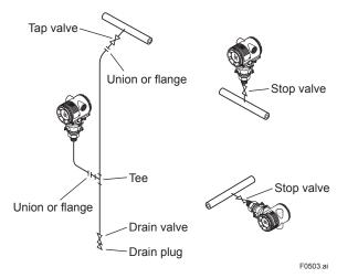
Figure 5.3 Impulse Piping Connection Examples
