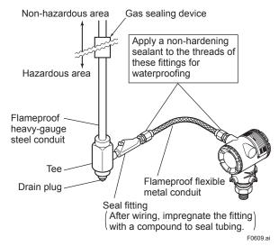
Figure 6.9 Typical Wiring Using Flameproof Metal Conduit
