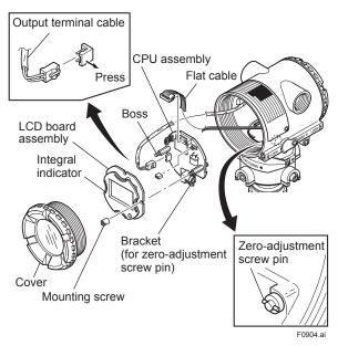
Figure 9.4 Removing and Attaching LCD Board Assembly and CPU Assembly
