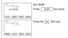
Note: Enter 0.00 to J15: SPAN ADJ to reset the span adjustment to the initial value at the shipment.
