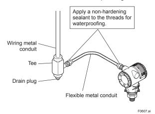
Figure 6.7 Typical Wiring Using Flexible Metal Conduit
