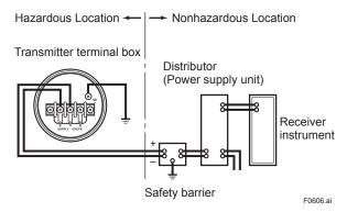
Figure 6.6 Connection between Transmitter and Distributor
