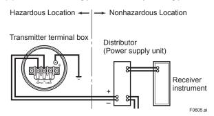
Figure 6.5 Connection between Transmitter and Distributor
