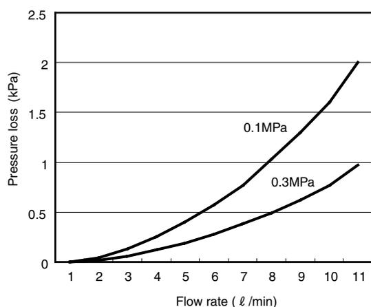
● If fiber tube is used, pressure loss may increase depended with piping condition. Care must be taken.
