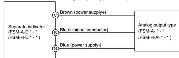
(Note) In metal body (stainless steel body and aluminum body) types, connect F.G. of equipment connected to - or + power supply to the body. Do not attempt insulation resistance and pressure tests while F.G. is connected, or may result in damage or burn.
