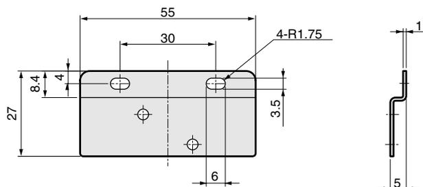
With M3 (length 6mm) 4 set screws for fixing
