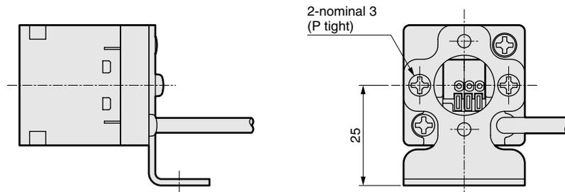
This bracket can be installed per 90 deg. increment against the switch body. Determine the installation attitude according to the location.
