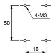
Bracket model no.: PPD3-KHS-D : Panel mount bracket set with panel cover
