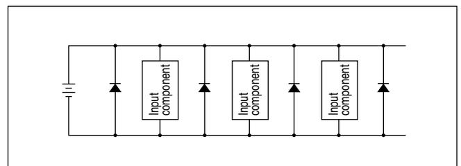
If components are connected with connectors, when the connector is removed while energized, the output circuit may be damaged. So, always mount or dismount the connector after the power is turned off.
