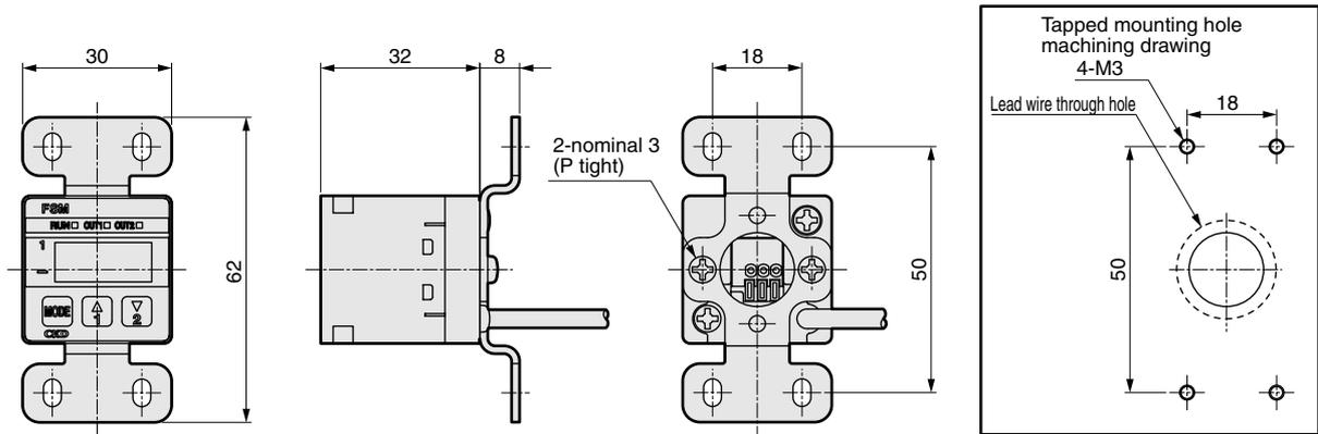
This bracket can be installed per 90 deg. increment.
