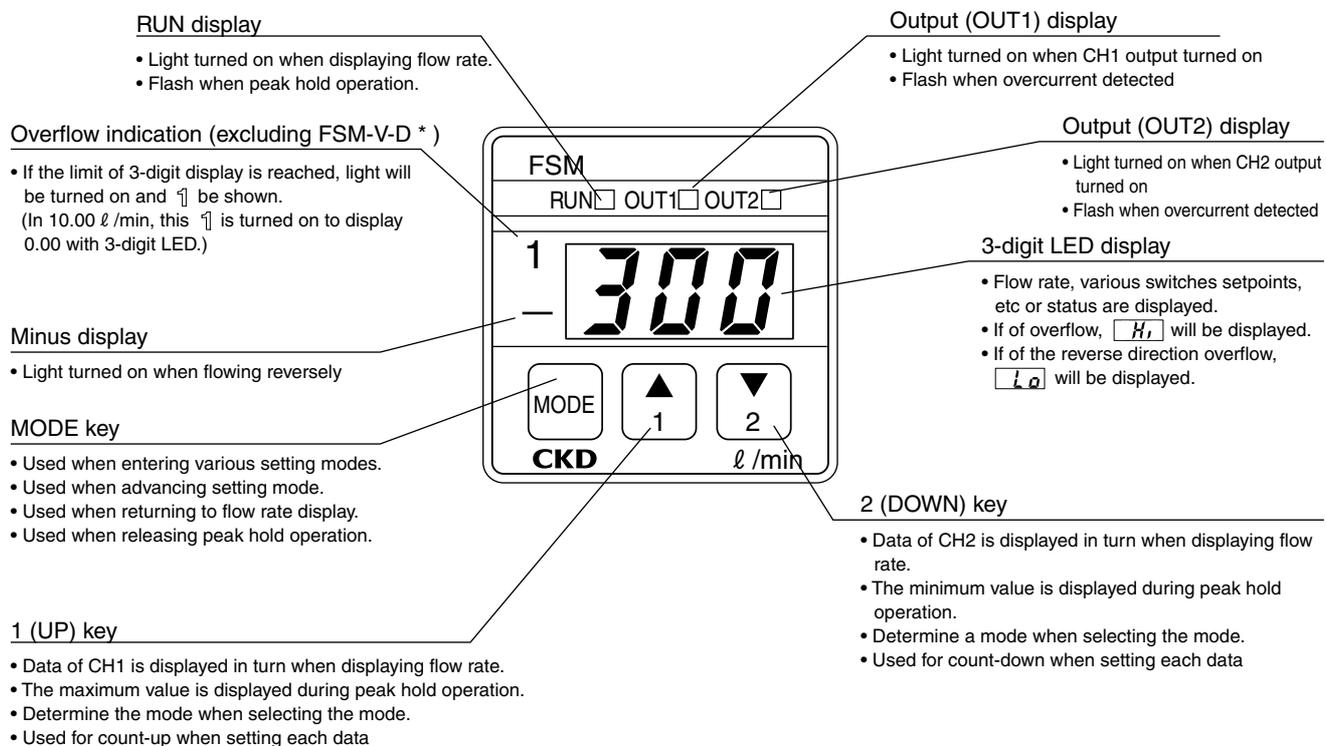
\*In FSM-H series, the design of front sheet differs. Name and functions of same display/controls are used.
